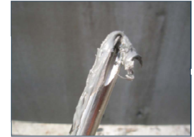
Wet epoxy component extracted from bridge hole 200
